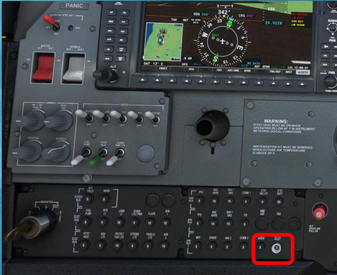
This doesn't work in the sim but good to know. If AP problems, recycle the white avionics power switches or red Masters.
